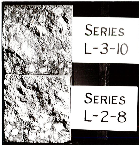
Figure 11. Failure surfaces of Series L-2 and L-3
