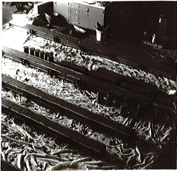
Figure 4. Finished beams and cylinders
